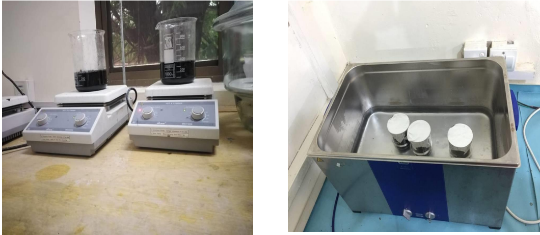
Figure 1: (a) Stirrer mechanism; (b) Bath sonicator
