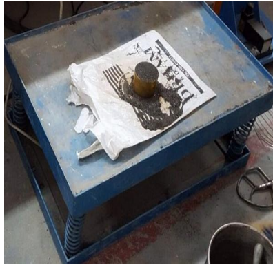
Figure 1: Determination of packing density using vibrating table
