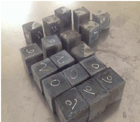
Figure 2: Samples of HSC before compressive strength testing
