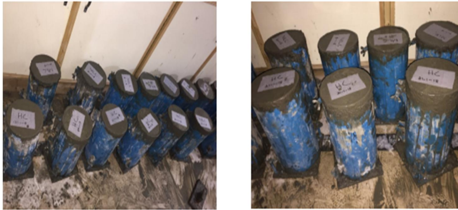
Figure 4: Casting of Test Specimens
