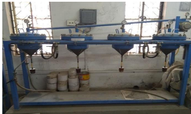
Figure 5: Water Permeability Test apparatus
