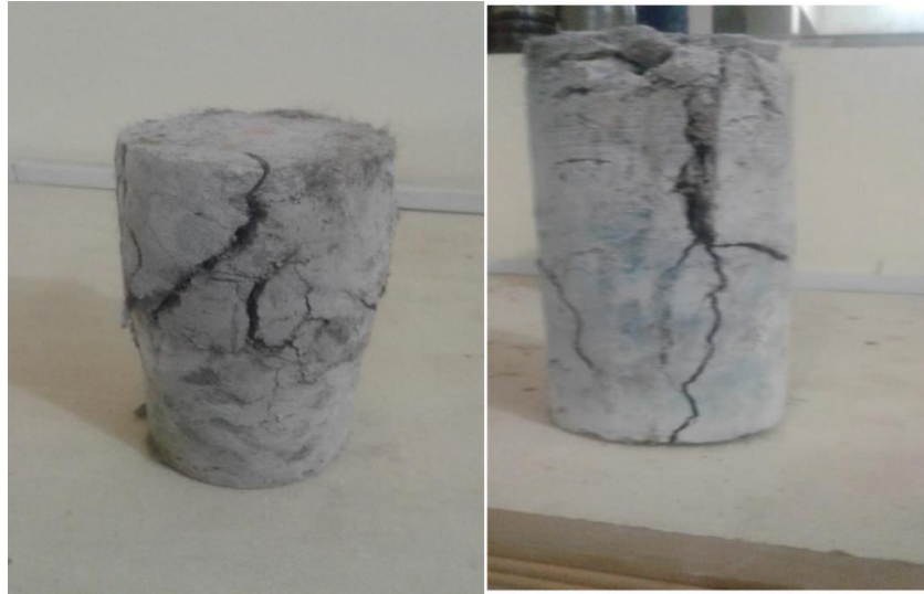
Figure 2: Failure pattern of concrete cylinders
