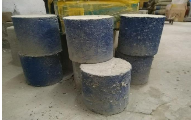
Figure 6: Application of Blue Emulsion paint to prevent penetration of water from sides
