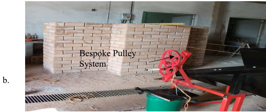
Figure. 3: Non-straight wall testing: (a) Schematic figure and (b) Test setup displaying system for lateral load
