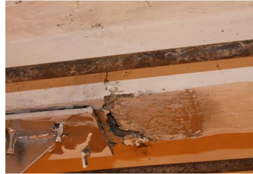
Figure 6: Damage in joint of as-built frame Figure 7: Flexure cracking in beam of retrofitted frame.
