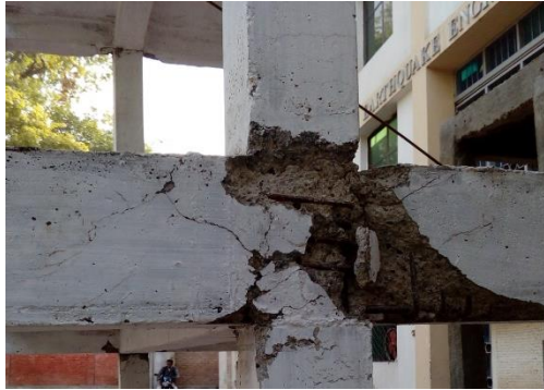
Figure 6: Damage in joint of as-built frame Figure 7: Flexure cracking in beam of retrofitted frame.
