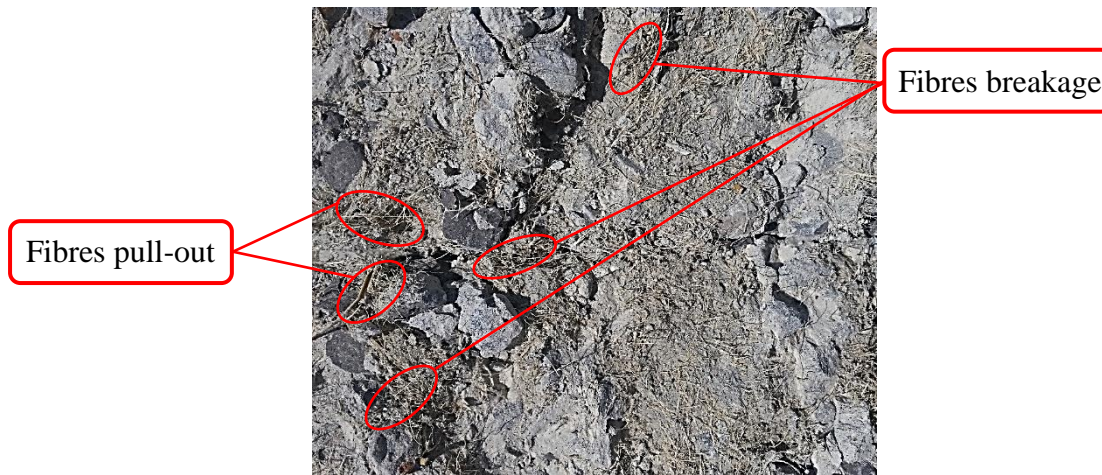
Figure 4: Fibres breakage and pull-out behavior
