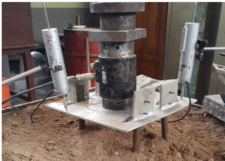
Figure 2: Instrumentation of Pile Group Model
