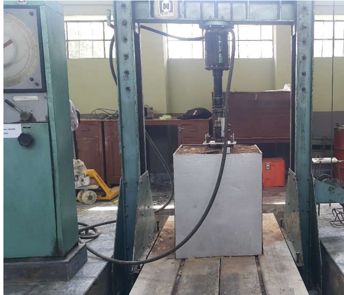
Figure 3: Loading strain frame
